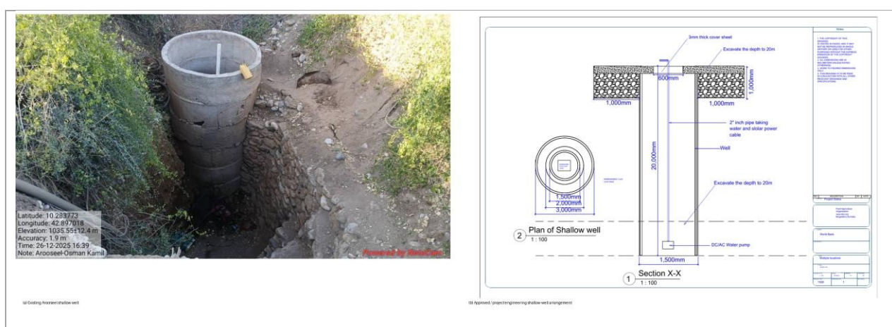
Figure 5-4: Representative Zeila Shallow-Well Condition and Rehabilitation Arrangement
